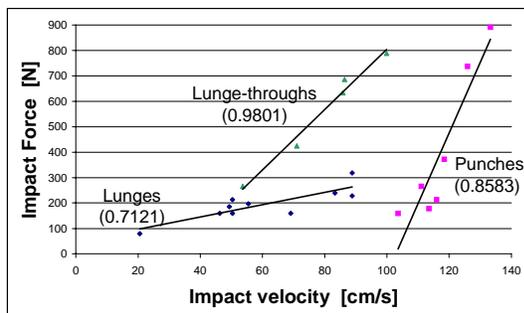
Figure 2. Comparison of impact velocity versus force for the three types of straight hits. ( $R^2$  values indicated)
