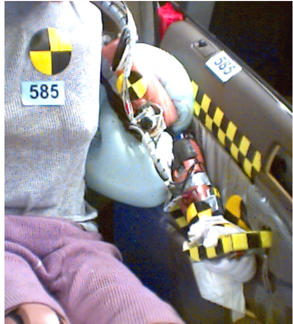
Figure 1. Oblique view of the side air bag loading the upper extremity 15 ms after deployment initiation.
