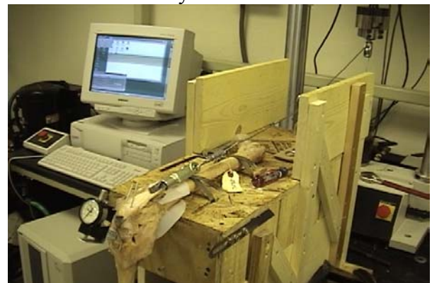
Figure 2: Specimen setup, showing the extensometer placement and the cable-and-pulley system assembly used to apply load to quadriceps tendon.
