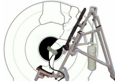
Figure 1: MR compatible back rest allows subject to assume ~0.45 body weight of load per knee.
