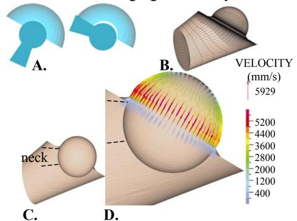
**Figure 1.** 3D CFD model (frontal view for a right hip). A. Schematic indicating sublaxation. B. Outer model view with visible mesh. C. Transparent view of the model with visible femoral head surface. D. Fluid velocity vectors at the beginning of the sublaxation for a 28 mm femoral head.
