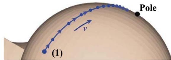
**Figure 3.** Pathline for fluid beginning at location (1) during the leg-cross subluxation. Each dot along the pathline indicates the position of the fluid for successive time points, in 0.001-second increments, up to the end of the subluxation (0.012 s).
