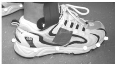
Figure 1. Ten markers (15 mm) affixed around the periphery of a running shoe were used to track insole sensor positions.
