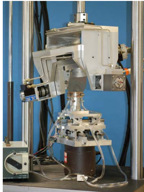
Figure 1: Total hip arthroplasty preparation in a multi-axis joint simulator, with third body particle circulation.
