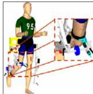
Figure 1: Experimental setup with limb in static posture. Series elastic elements allow for stimulation induced joint movements.
