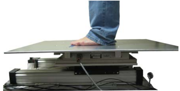
Figure 1: Experimental set-up of the PIMP. The PIMP translated a maximum of 0.15 m forward and 0.25 m backward at an average velocity of 0.45 m/s. A force platform is integrated with the PIMP and used to quantify balance.
