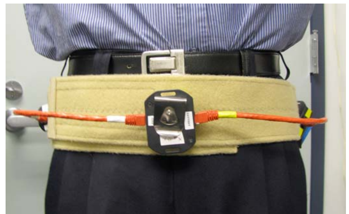
Figure 1: Accelerometer measurement system. Left: transmitter, middle: sensor, right: battery
