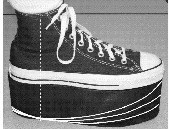
Figure 1: High top canvas shoe with stiff crepe material attached. Different radii were obtained by cutting along the lines drawn on the sole (lines in the picture are not drawn to scale).
