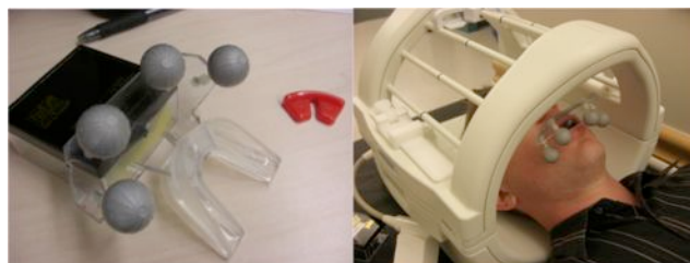
Figure 3: Custom mouthpiece / bite-bar for use in the MR environment.
