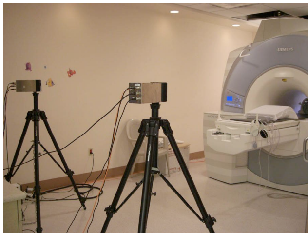
Figure 2: A.R.T. Track3 stereovision system and Siemens 3T scanner located in the MRI room.
