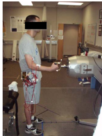
Figure 1: Instrumented subject holding dynamometer handle in testing position.
