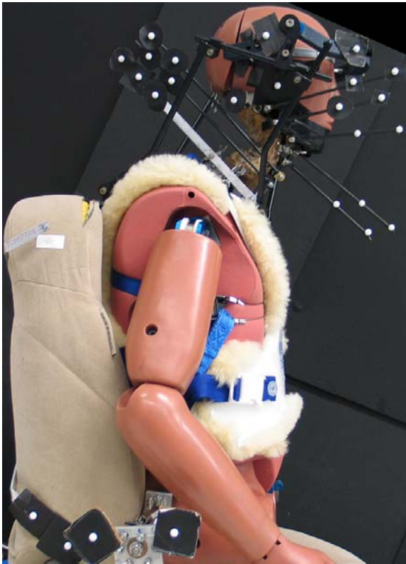
Fig. 1. Photograph of the Human Model of the Neck (HUMON) with the halo-vest. Motion tracking flags were fixed to the head, cervical vertebrae, and pelvis.
