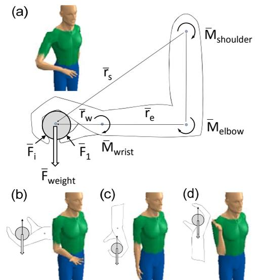
**Figure 1:** External forces and moments on upper limb joints in (a) overhand approach and finger grip; (b) underhand approach and palm grip; (c) holding cylinder at side of body using a hook grip (thigh height); and (d) holding cylinder with a vertical forearm using a palm grip at shoulder height.
