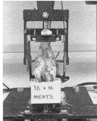
Figure 2: Porcine specimen mounted into the MTS loading fixture.
