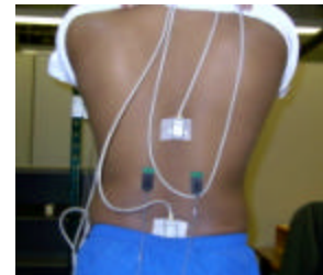
Figure 1: Three markers attached to participant over manubrium, T10 and S1 spinous process. The EMG electrodes are placed over the erector spinae muscle group at L2/L3 level of lumbar spine.
