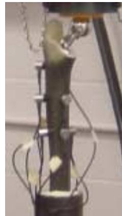
Fig. 1 THA specimen with eight sensors
