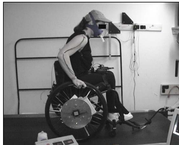
Figure 1. Demand on the user was measured using a propulsimeter, a portable gas analyzer, and a heart rate monitor.
