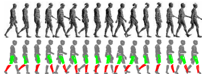
Figure 2: Visual hulls constructed using 7 cameras (top). Articulated body matched to visual hulls (bottom).
