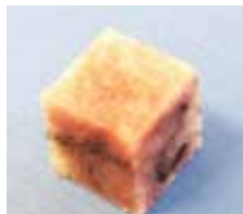
Figure 1: Photograph of a cubic bone specimen which was cut from a canine femoral head
