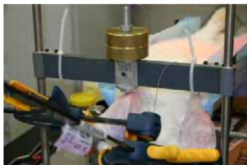
Figure 1: Impact set-up showing impactor in approximation to the rabbit's patella.
