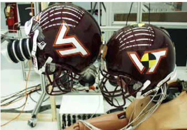
Figure 1: The impacted helmet was mounted to a HIII headform and neck and then to a full HIII body.
