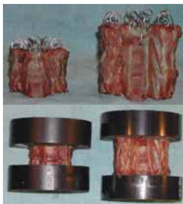
Figure 1: Human Cervical Spine C3-C5 Segments Prepared for Testing. A 5-year old (left) and 18-year old (right) are shown wired on top and embedded in PMMA for testing (bottom).
