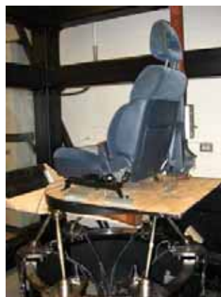
Figure 1: Automobile seat mounted on robotic platform. The platform motion has been programmed to simulate whiplash-like perturbations.
