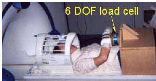
Figure 1: Subject position and load cell mounting setup used during function MRI sessions.
