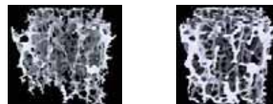
Figure 1: Scaled version of a normal (right) and osteopenic (left) bone cubes were made using rapid prototyping system.
