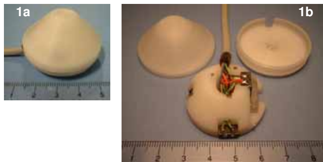
Figure 1: (a) one 3D gyroscope unit, (b) components of the plastic housing.
