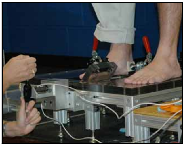
Figure 1: A subject's foot was loaded in inversion using the proposed Barefoot Torsional Flexibility Device.
