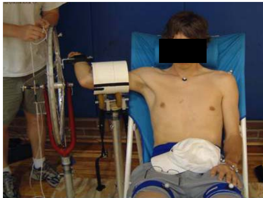
Figure 2: The researcher slowly pulled on a rope to externally rotate the subject's arm. The rope ran through a pulley that was attached to a load cell (to measure rotational resistance). A potentiometer was mounted to the bicycle wheel (to measure ROM).
