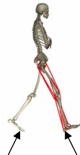
Figure 1: Planar, seven-segment, nine-degree of freedom musculoskeletal model.
