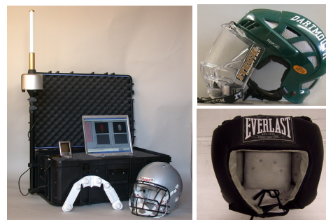
Figure 1: Instrumented football, hockey, and boxing helmets
