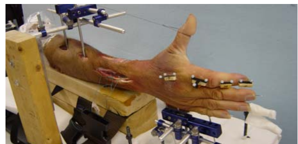
Figure 1: A cadaver hand mounted on a custom fixation device for tendon loading and motion recording.
