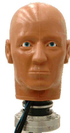
Figure 2: The FOCUS headform is designed to predict eye and facial injuries.
