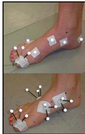
Figure 1: A) Point markers attached to the segments of the foot (one on hindfoot and one on midfoot not shown) B) Triad clusters attached to the segments of the foot (one on hindfoot not shown).
