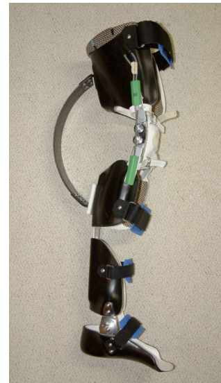
Figure 1: Knee orthosis with carbon composite leaf spring on posterior side for energy storage during knee flexion. Ankle joint is free-moving and passive.
