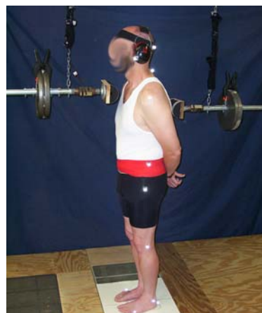
Figure 1: Participants stood relaxed with their eyes closed. Perturbations were administered with two padded and weighted ballistic pendulums placed both in front of and behind the participant
