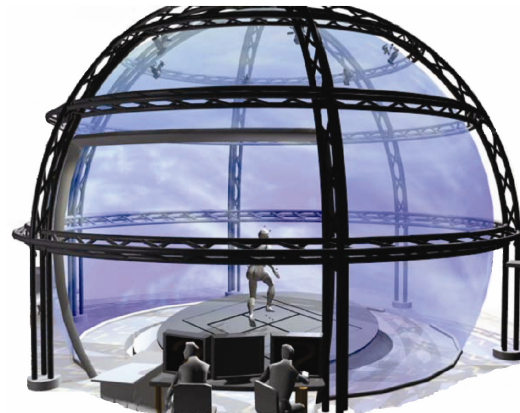
Fig. 1. The CAREN at CFI is an immersive VR system contained in a 7m diameter dome with a six degree of freedom platform with a built-in instrumented treadmill.
