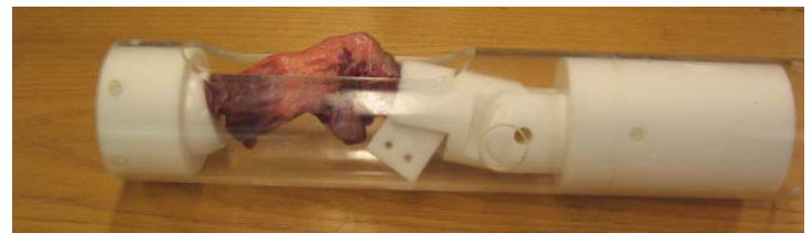
Figure 1. Device used to apply physiologic loads to a secured ovine stifle joint at various flexion angles
