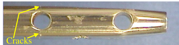
Figure 3: Representative failure of tibial nail: distal segment
