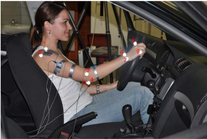
Figure 2: EMG and kinematic data collection during gear shifting.
