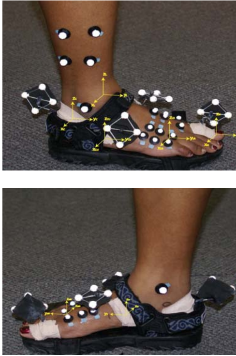
Figure 1: Technical and anatomical markers. Top figure: Leg ( x_L, y_L, z_L ), calcaneus ( x_C, y_C, z_C ), cuboid ( x_{CU}, y_{CU}, z_{CU} ), lateral rays ( x_{LR}, y_{LR}, z_{LR} ), and hallux ( x_H, y_H, z_H ) anatomical coordinate systems. Bottom figure: Navicular ( x_N, y_N, z_N ), and medial rays ( x_{MR}, y_{MR}, z_{MR} ) anatomical coordinate systems. All of the anatomical coordinate systems were defined using the appropriate anatomical landmarks
