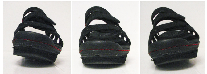
Figure 1: The perturbing shoe showing undeveloped fulcrum (middle), medially deployed fulcrum that inverts during midstance (left), and laterally deployed fulcrum that everts during midstance (right).
