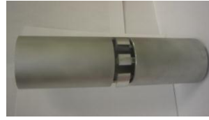
Fig. 3 Custom-made circular dynamometer
