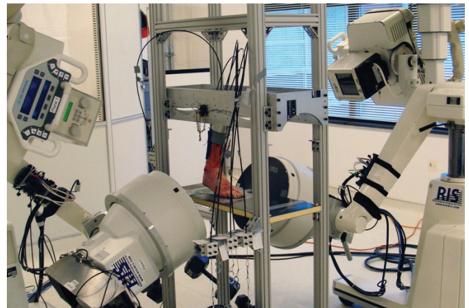
Figure 1: Apparatus within the XROMM system, with 2 x-rays oblique to the lateral aspect of the foot.
