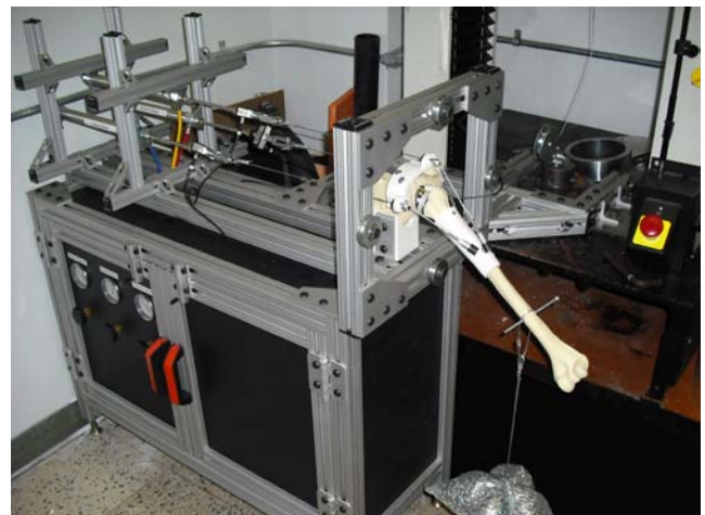
Figure 1: Mechanical shoulder simulator
