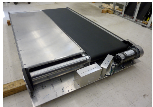
Figure 3: Treadmills placed side-by-side. The belt and motor of the left treadmill have been removed to expose the rollers and light-weight deck.
