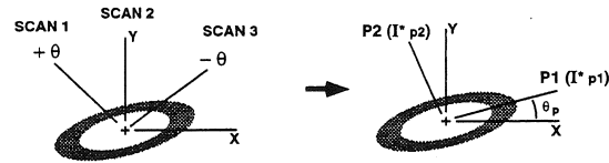
Figure 2: Principal moments of inertia ( I_{min} , I_{max} ) and orientations of principal axes ( \theta_p , \theta_p + 90^\circ ) are determined from independent analyses of 3 scans.
