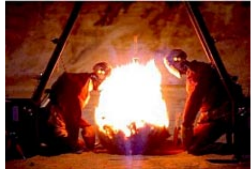
Figure 1: Simulated Antipersonnel Mine Blast with Hybrid III Surrogates
