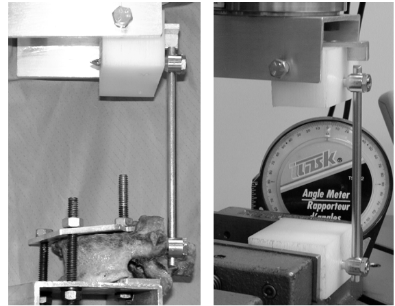
Figure 1: Test setup used to compare motion of pedicle screw in bone and in UHMWPE.
