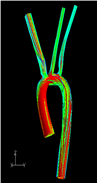
Fig.1 Simulated blood flow in the human aorta using an overset mesh technique.
