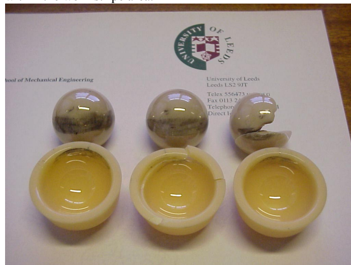
Figure 1. Fractured Alumina Insert (Middle) and Zirconia Head (right) after severe microseparation.
