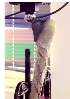
Figure 2: The strain measurement of C-S prosthetic femora.
