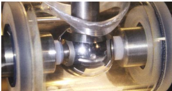
Figure 1: Pin-on-ball testing device.
