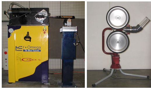
Figure 1: Blunt Impactor (left), and Pitching Machine (right)
