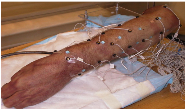
Figure 1: Surface markers on the upper limb specimen
