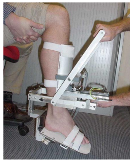
Figure 2. Quasi static ankle tester
