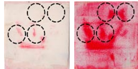
Figure 2: Medium (left) and Low (right) Fuji film results, dotted lines show position of FlexiForce sensors
