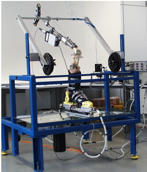
Figure 1: Device to apply external loads and quadriceps forces to cadaver knee joints with simultaneous measurement of ski binding forces and moments.
