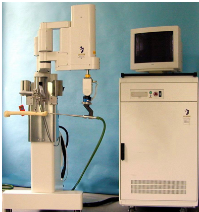
Figure 1: The control computer together with the ROBODOC® robot with 5 degrees of freedom. The pneumatic turbine with the reamers bearing sleeve is attached to the robot arm.
