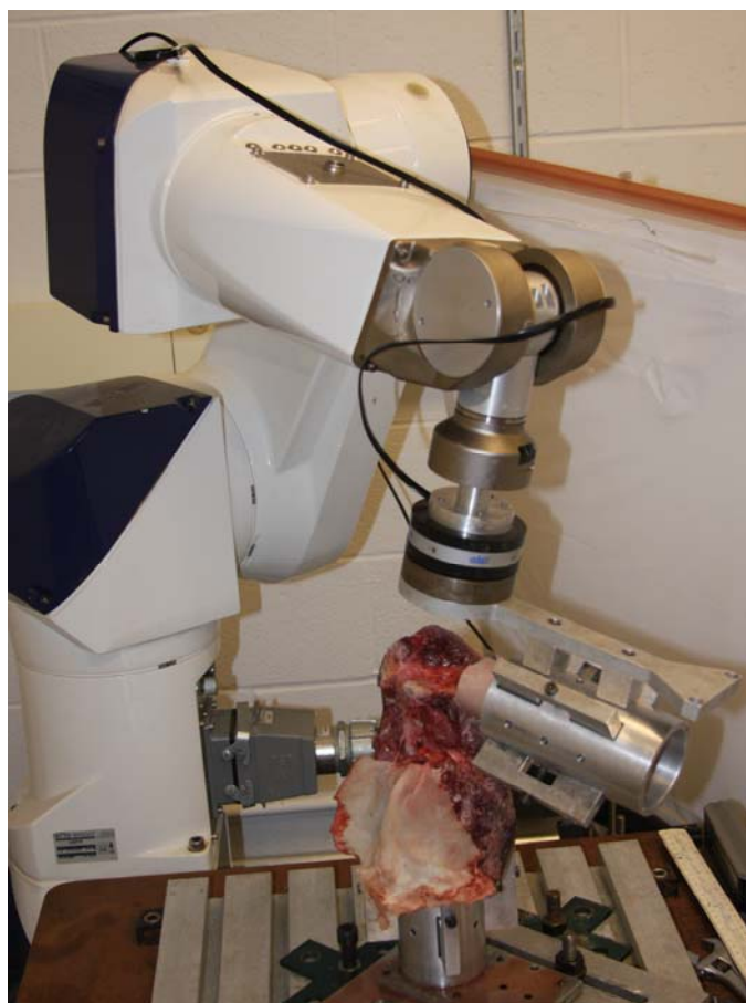
Figure 1: Elbow specimen mounted in robot manipulator
