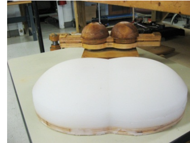
Figure 1. Foreground: Elastomeric gel buttocks model. Background: rigid substructure.
