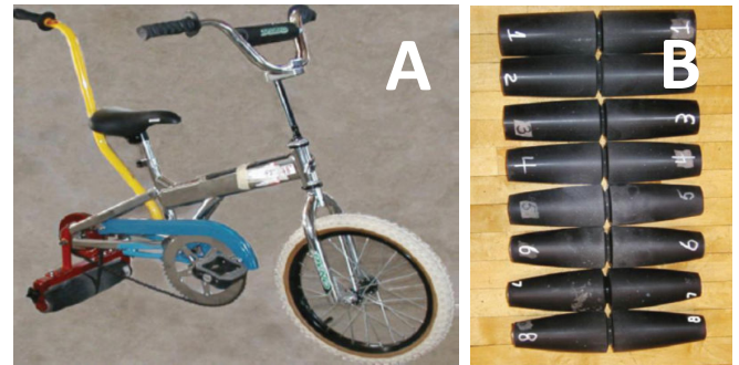
Figure 1: (A) The adapted bicycles used by Lose the Training Wheels utilize crowned rollers in place of a rear wheel. (B) The most crowned roller (bottom) accentuates bicycle tipping.
