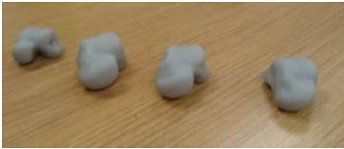
Figure 1: 3D prototype models of 4 different talus bones.
