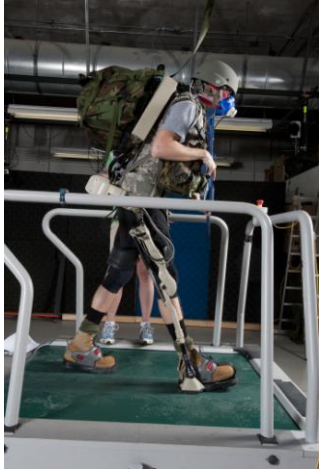
Figure 1: Soldier wearing the PEXO with the military load attached while walking on the treadmill at 1.34 m/s.
