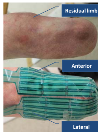
Figure 1. Residual limb with F-socket sensor.
