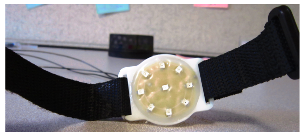
Figure 1: Photograph of beta prototype, which includes a ring of sensors, conformable gel, and housing with adjustable strap.
