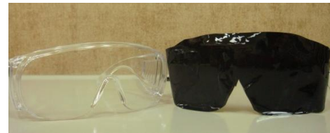
Figure 2: The clear goggles used as control condition (left) and goggles attached with 2-layered window films to reduce light intensity (right).
