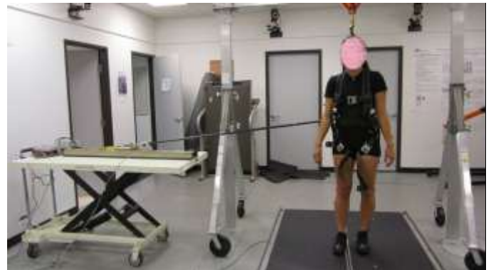
Figure 1. Experiment setup with participant standing on a split-belt treadmill, attached to the linear motor, and secured to a gantry for safety. The linear motor was mounted to the left on the scissor table.
