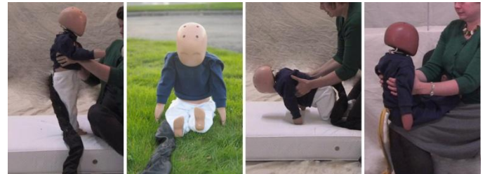
Figure 1: CRABI ATD initial positions on the different test surfaces (head butt not shown).
