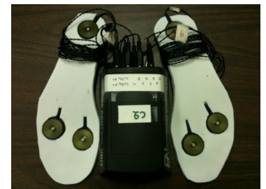
Figure 1. The vibrotactile stimulation system.
