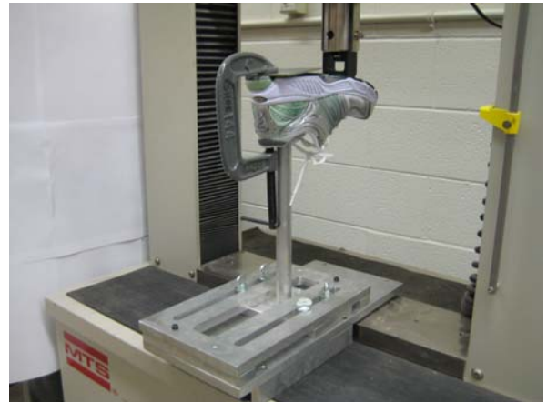
Figure 1: Testing apparatus with adjustable base and experimental setup in the MTS machine [4]
