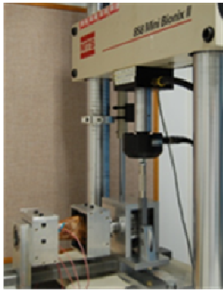
Figure 2. Linear actuated torsional device with potted cadaveric specimen.
