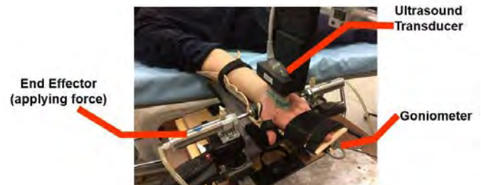
Figure 1. Experimental setup of in vivo ultrasound imaging
