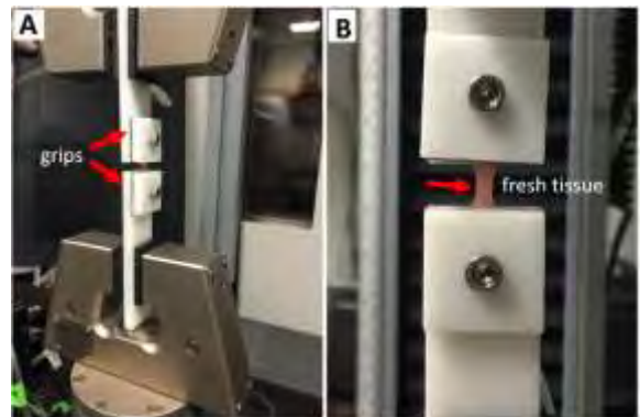
Figure 1: Tensile test performed using an Instron type 5565 with anti-slip grips.
