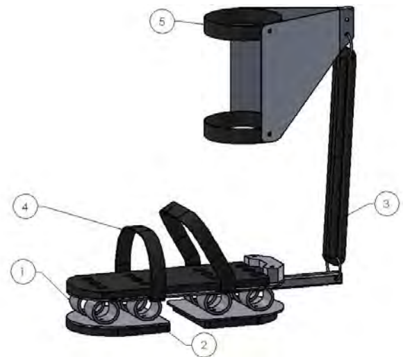
Figure 2: CAD model of the proposed device. (Components: 1 - Compressive elastic elements, 2 - Separated sole, 3 - Tensile elastic element, 4 - Shoe straps, and 5 - Calf straps)
