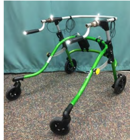
Figure 1: Instrumented walker with five markers (left/right grip, left/right load cell, bar) and load cells at connection from handles to walker.
