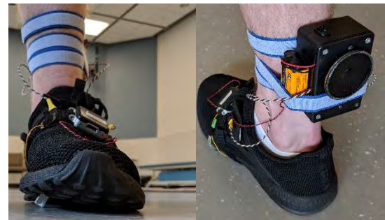
Figure 1: Left: The aluminum flap creating an inversion of the ankle. Right: The controller, containing a speaker, was strapped on the shank above the ankle.
