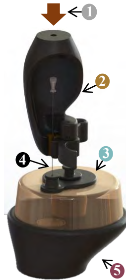
Figure 1. Test fixture diagram. 1) Force applied by MTS. 2) Needle grip that simulates physician's grip. 3) Ballistics gelatin tissue surrogate. 4) Needle. 5) Barrier.
