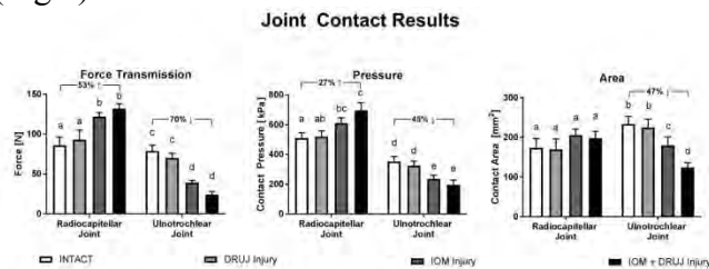
Figure 2: Mean force, contact pressure, and contact area at the elbow joint in pronation under the four testing conditions. RC: radiocapitellar, UT: ulnotrochlear. Lowercase letters represent the result of Least Squares post-hoc comparisons within either the radiocapitellar or ulnotrochlear regions ( p < 0.05 ). Columns with a letter in common are not statistically different from one another (i.e. p > 0.05 ). Where statistically significant differences were detected between the INTACT and IOM + DRUJ Injury groups, relative percent increases (%↑) and decreases (%↓) are indicated.
